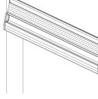
Mount the brackets 50mm from each end of the rail. All brackets must be aligned and evenly spaced when more than two brackets are required. Space Evenly 50 mm
